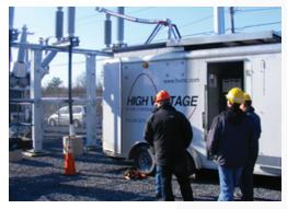
The below design includes a PD & TD cable diagnostic testing package (customer fabricated test truck)
