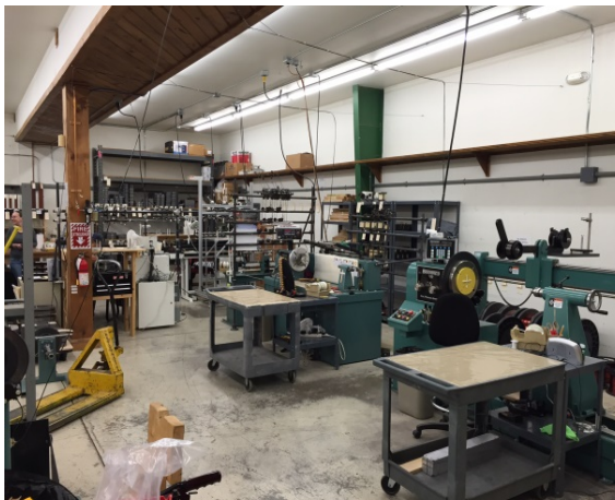
Five multi-winding and two hand winding machines
