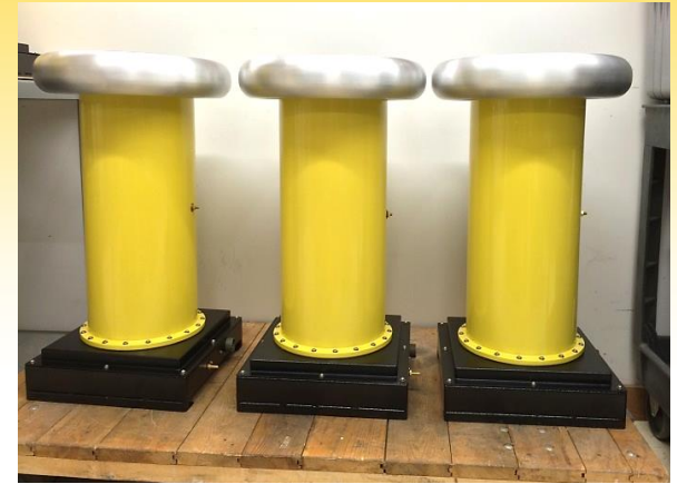
Fiberglass tubes containing transformers, oil filled A look inside - below picture
