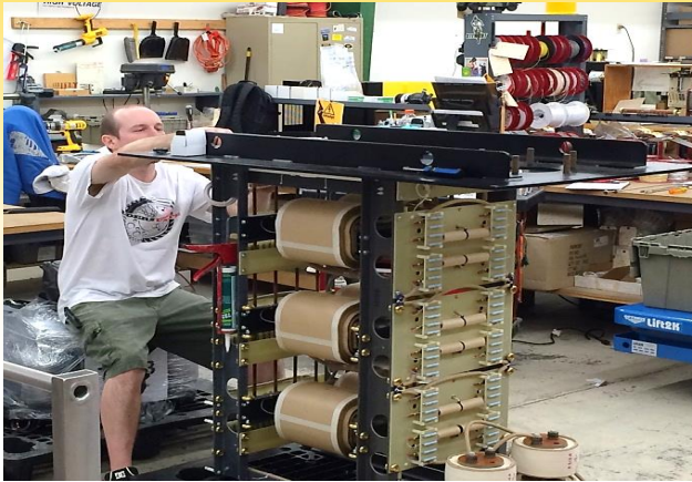
Tank building in process: transformers, rectifiers, resistors, solenoids, capacitors, bushings, ...
