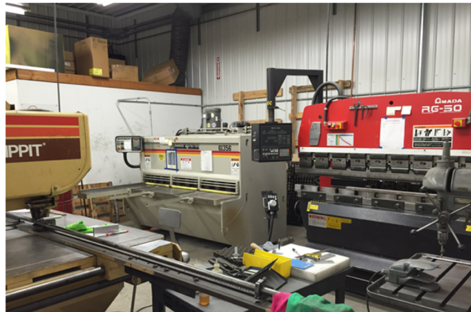
Steel & aluminum cabinet and oil tank production using metal shears, punches, breaks and Stripit machines
