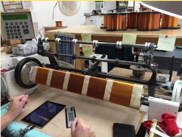
Multi-winding five transformers at a time
